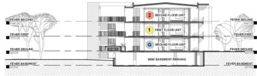
FEVER BLOCK - TYPICAL SECTION SCALE 1 : 200
